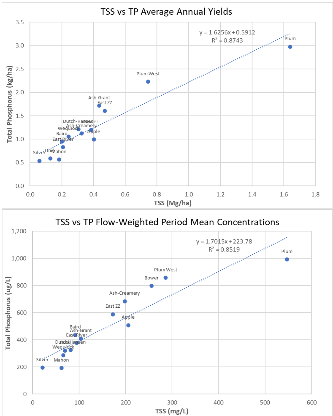
Figure 13. Average annual yield relationships between TSS and total phosphorus (upper) are compared to flow-weighted period mean concentration relationships (lower) at intensive stations in L. Fox sub-basin. The flow-weighted concentrations in the lower figure are typically better for site comparisons because they greatly reduce the variation caused by large fluctuations of annual discharge, especially when the monitoring periods are different (or precipitation is quite different). For example, average annual discharge was 164 mm at Ashwaubenon Creamery road station (2004-2006), compared to 419 mm at Ashwaubenon Hansen road station (2019-2021).
