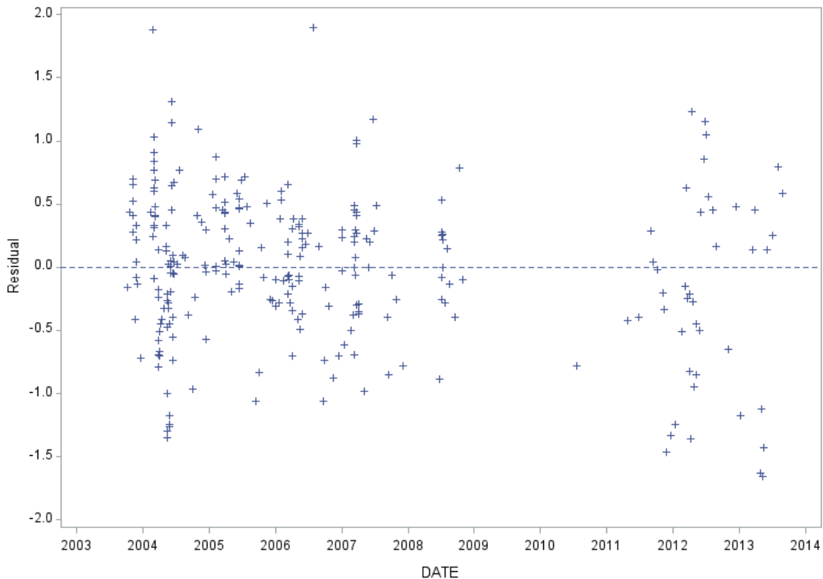
Figure 5. Flow and seasonally-adjusted residuals of log-transformed TP during Periods 3 and 4 (water years 2004-2013). Note the slight downward trend over time ( p = 0.0019 for date).
