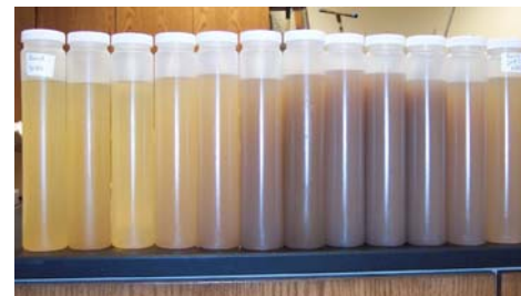
ISCO sample bottles showing changes in sediment concentrations over an event hydrograph
