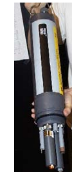
YSI-6200 sonde and example dissolved oxygen data from fall 2003.
