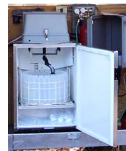
24 1-liter samples can be collected before servicing
