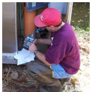
Accessing the data logger
