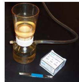
Filtering a sample for dissolved phosphorus
