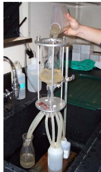
Splitting an ISCO sample bottle into SSC, TSS, and total phosphorus subsamples using a Teflon cone splitter
