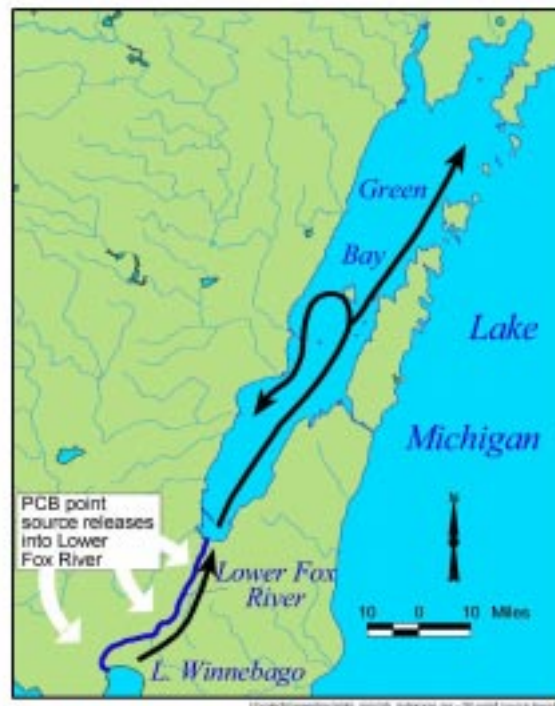
Figure 2.6. The movement of PCBs from the Lower Fox River throughout Green Bay. Water circulation patterns in the river and bay determine the movement of the PCBs.
