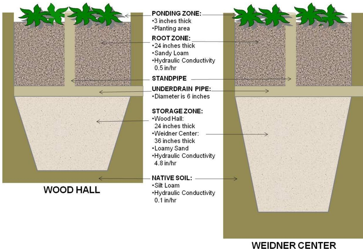
**Figure 3.11: Selected designs for bioretention cells**
