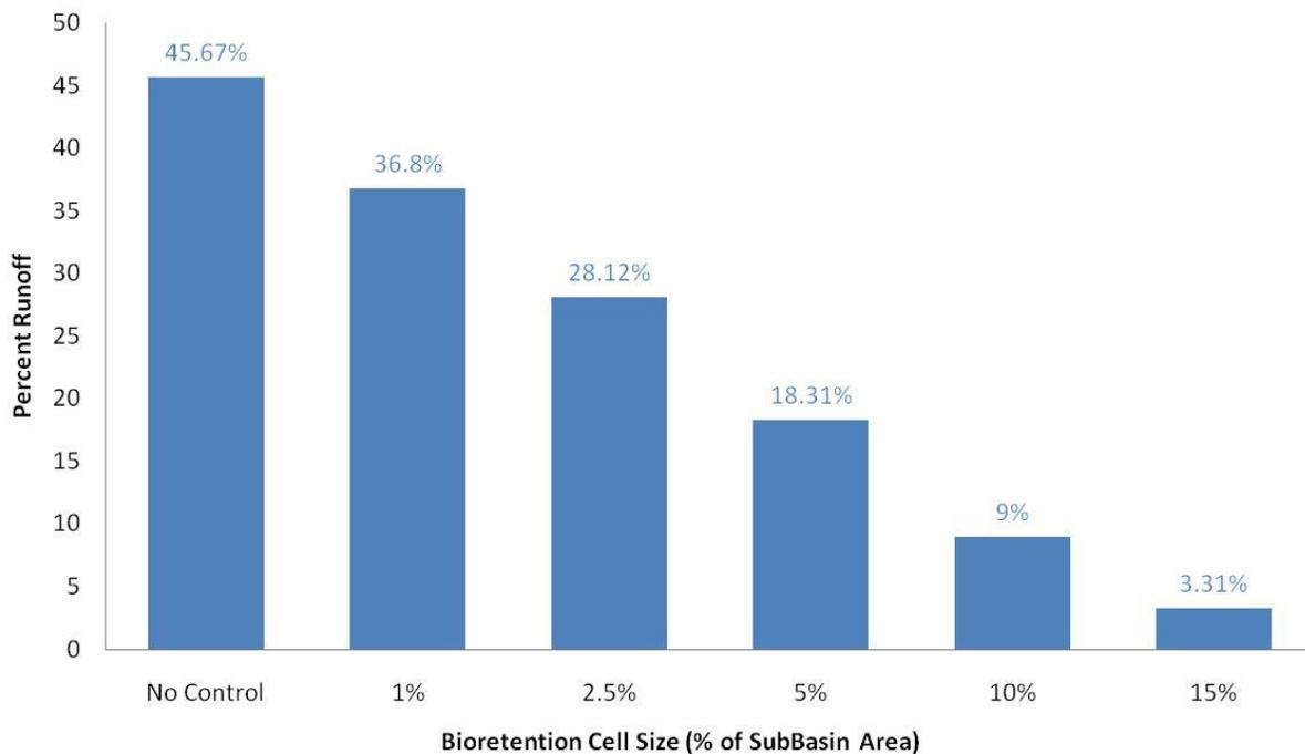
**Figure 3.10: Percent of runoff leaving the Weidner Center sub-basin for different size bioretention cells.**
