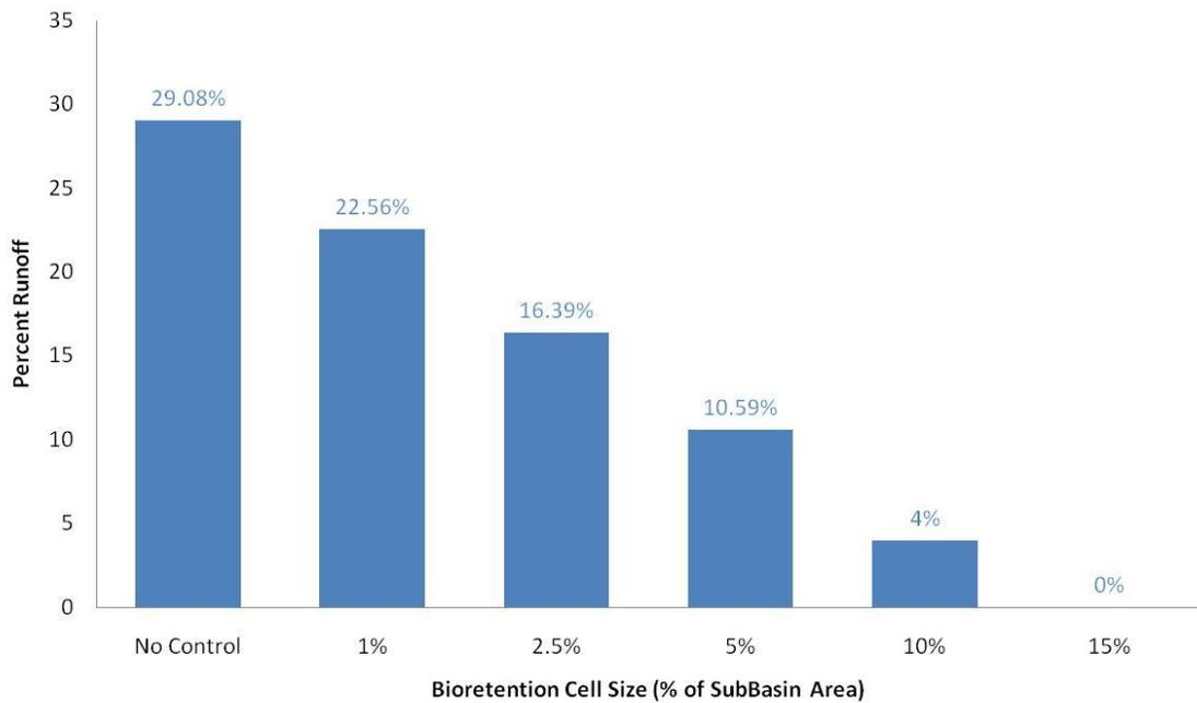
**Figure 3.9: Percent of runoff leaving the Wood Hall sub-basin for different size bioretention cells.**
