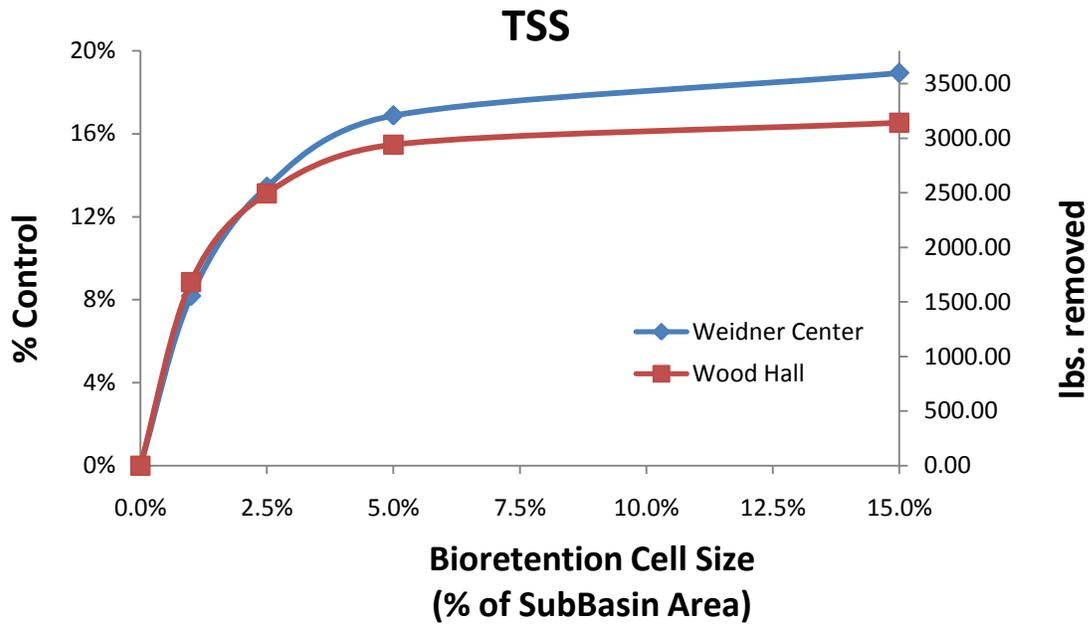
Figure 2. Percent of TSS control and lbs. of TSS removed from 4 sizes of bioretention devices in the Weidner Center sub-basin and Wood Hall sub-basin. Results reflect pollutant reduction within the entire Basin 15.
