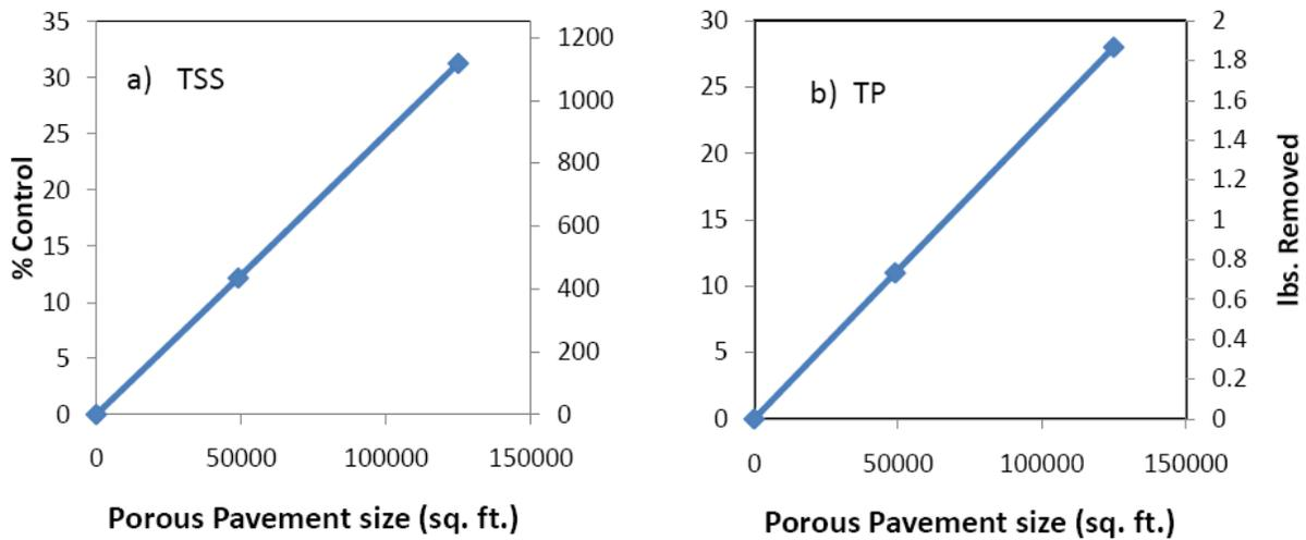
Figure 4. Percent control (primary axis) and lbs. removed (secondary axis) of a) TSS and b) TP for the porous pavement scenarios.
