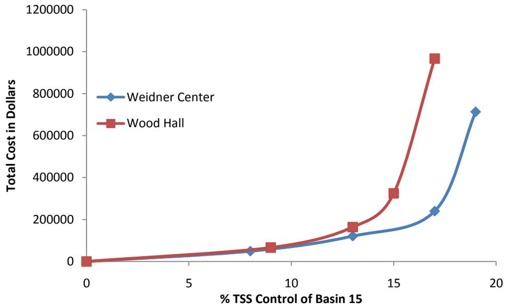
Figure 5. Total cost of each bioretention cell plotted against the percent Total Suspended Solids (TSS) for Basin 15. Data points are each size (1%, 2.5%, 5%, and 15% of the total area of each contributing sub-basin).
