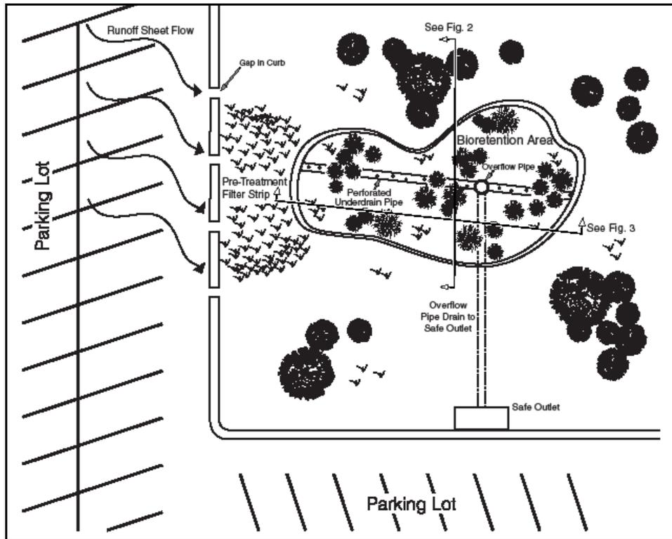
**Figure 3.5: Typical layout of a bioretention cell capturing runoff from a parking lot (WDNR 2006)**
