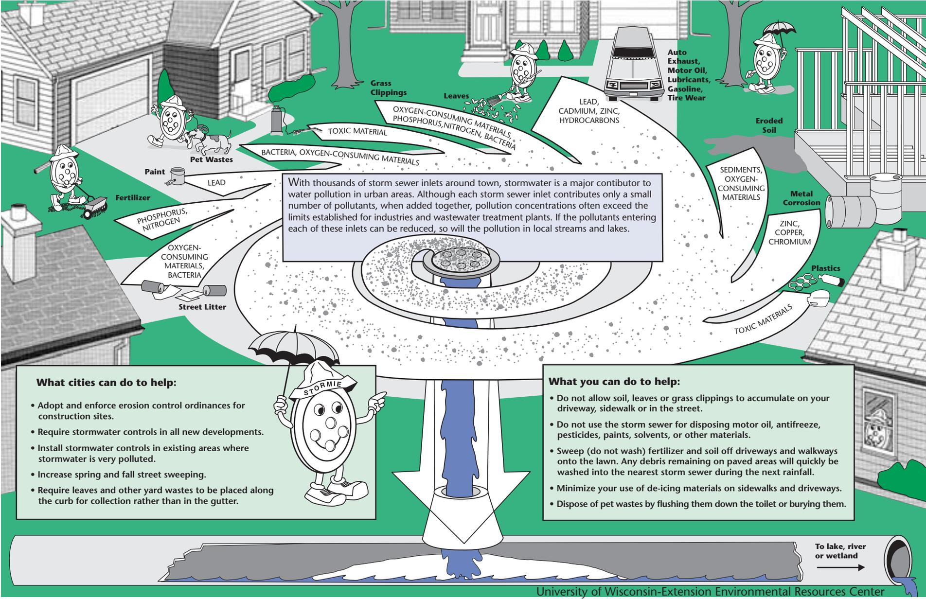
With thousands of storm sewer inlets around town, stormwater is a major contributor to water pollution in urban areas. Although each storm sewer inlet contributes only a small number of pollutants, when added together, pollution concentrations often exceed the limits established for industries and wastewater treatment plants. If the pollutants entering each of these inlets can be reduced, so will the pollution in local streams and lakes.
