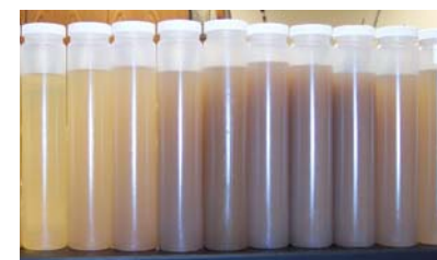
Figure 7. Event samples showing sediment concentration change during a storm.
