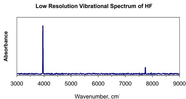
*This question requires the students to understand the concept that the two peaks correspond to a fundamental peak between vibrational levels  $n=0$  and  $n=1$ , while the overtone peak corresponds to a transition between the vibrational levels  $n=0$  and  $n=2$ . Knowing this they can use the given vibrational energy equation to calculate the vibrational constants (2 equations/2 unknowns).*
