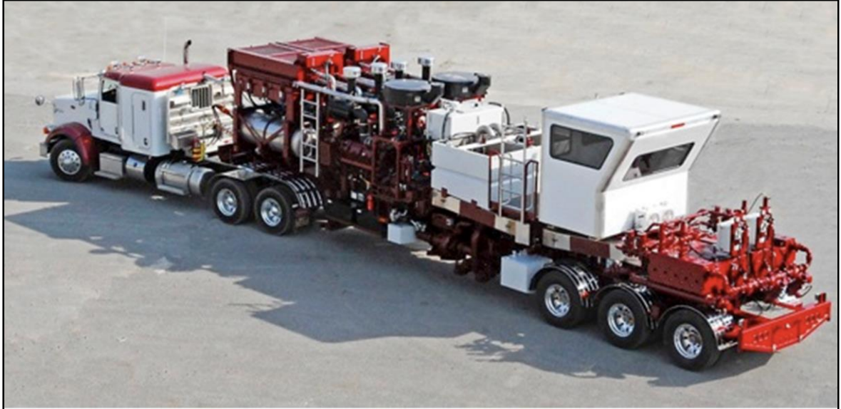
High-Pressure Pump (2000 HP; 15,000 psi; 20bpm)
