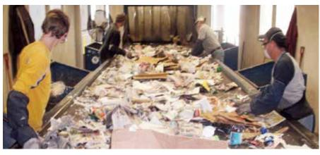
**PRE-SORT LINE:** The sorters remove items that may harm or interfere with equipment such as plastic bags, large metal items and trash.
