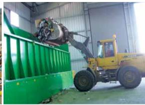
**METERING BIN:** This machine evenly meters the amount of recycling entering the facility.
