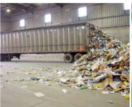
TIP FLOOR: The trucks empty recyclables onto the tipping floor.
