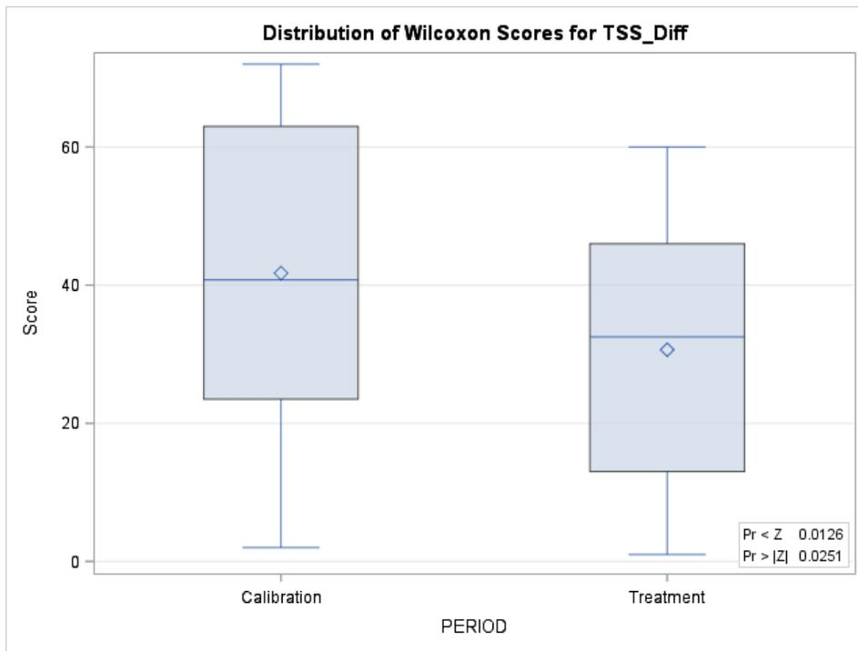
Figure 19. Boxplots of Wilcoxon scores for TSS during calibration (pre-treatment) and post-treatment periods. A significant decline in TSS during treatment phase is indicated ( $p < 0.05$ ).
