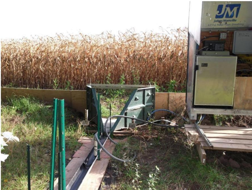
Figure 3. Station housing and monitoring equipment at outlet of west catchment. Turbidity probe is mounted below flume in half-pipe.
