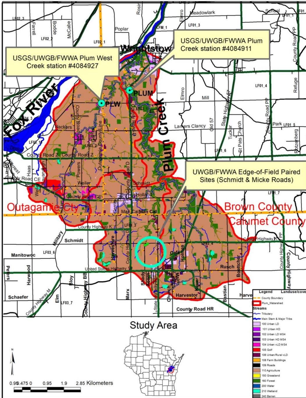
Figure 1. Plum Creek watershed and location of paired edge-of-field monitoring stations. Two USGS water quality monitoring stations that were also funded through the GLRI Fox-Wolf Watershed Alliance project are shown for reference.
