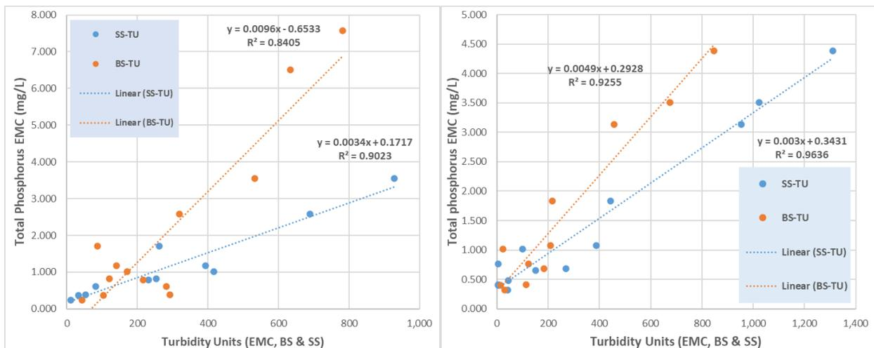
Figure 15. Backscatter (BS-TU) and sidescatter (SS-TU) turbidity units compared to total phosphorus concentrations, on an event-mean basis. North station (left) and south station (right) at Oneida grazing study site.
