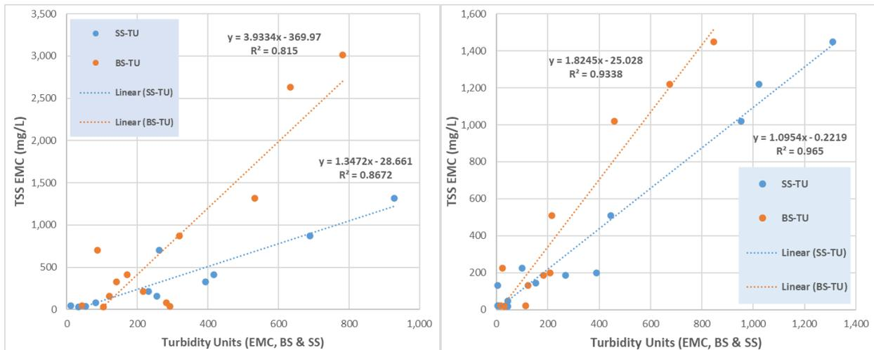
Figure 14. Backscatter (BS-TU) and sidescatter (SS-TU) turbidity units compared to TSS concentrations, on an event-mean basis. North station (left) and south station (right) at Oneida grazing study site.
