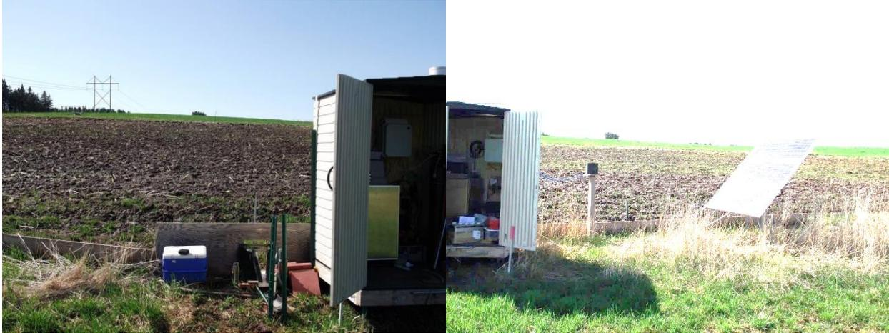
*Figure 4. Station housing and monitoring equipment at outlet of south catchment (left, 5/5/18) and north catchment (right). Turbidity probe is mounted below flume in half-pipe.*
