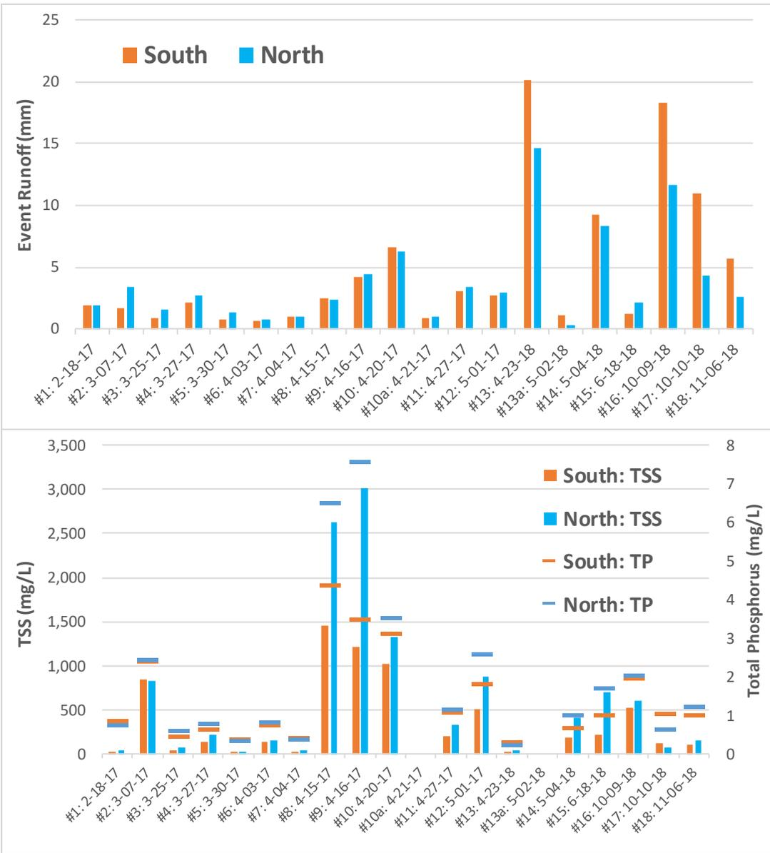
Figure 10. Area-weighted runoff volume (upper, in mm), and event-mean concentrations of TSS and total phosphorus (lower, in mg/L) by event for south and north paired catchments during pre-treatment period.
