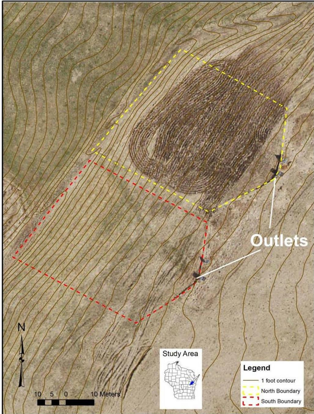
Figure 3. Study site with paired north and south catchment boundaries, and 1 foot contours. Monitoring station houses, wingwalls and solar panels can be seen in April 2021 aerial ortho-photo. The tillage pattern from the fall 2020 chisel plow operation can be seen in the north catchment. One foot elevation contours (2018 LIDAR) and background 2021 aerial ortho-photo are from the Outagamie County Land Information Office.
