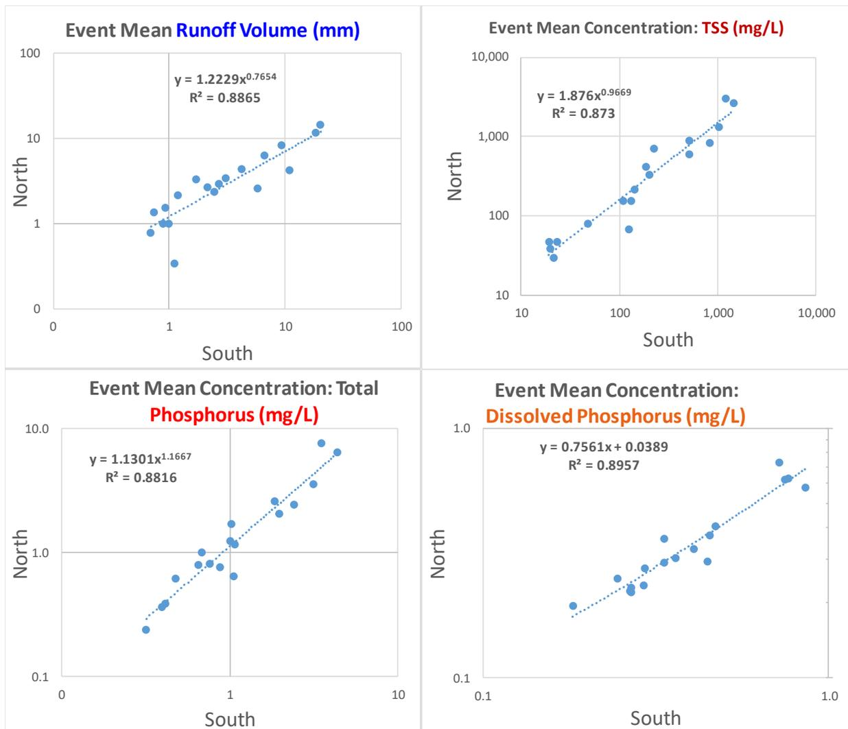
Figure 12. Log-space regression plots of South and North paired EOF catchments for runoff volume ( $n=20$ ), and event-mean concentrations of TSS ( $n=18$ ), TP ( $n=18$ ) and DP ( $n=18$ ) during 20 calibration (pre-treatment) period events.
