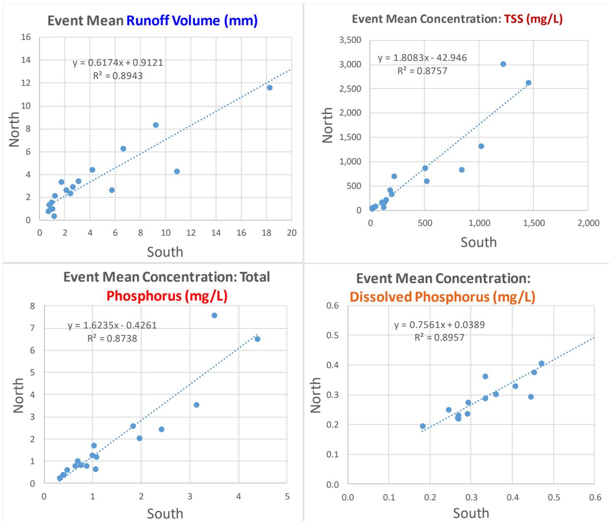
Figure 11. Regression plots of South and North paired EOF catchments for runoff volume ( $n=20$ ), and event-mean concentrations of TSS ( $n=18$ ), TP ( $n=18$ ) and DP ( $n=18$ ) during 20 calibration (pre-treatment) period events.
