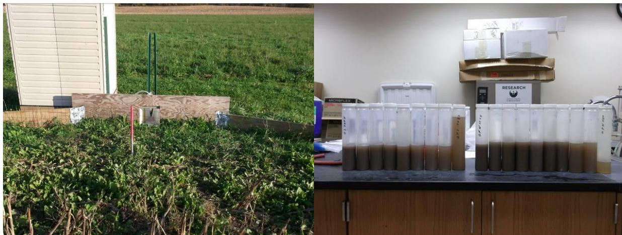
*Figure 5. Photo view looking downslope toward north station plywood berms and 1' H-flume, with trash fence just upslope of flume to prevent clogging of narrow flume outlet by debris (left, 10/22/16). Image on right of south and north station automated sampler bottles collected from 4/20/17 event and awaiting compositing and processing.*
