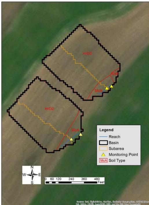
Figure 16. Watershed boundaries, subareas, water reaches, soils, and outlet points for Oneida North and South paired watersheds as modeled by Kalk (2018). Soil type map units are from the USDA SSURGO database.
