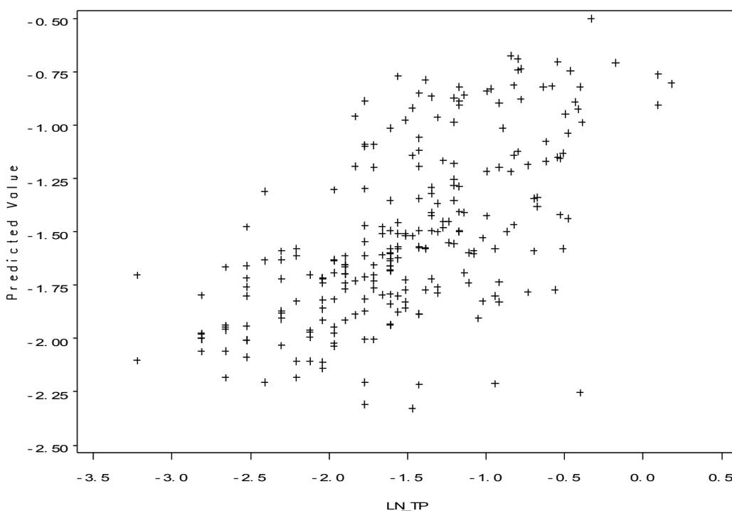
Figure 3.5. Observed and predicted log-transformed total phosphorus (LN\_TP) concentrations during Period 1 with the selected best fit regression model (adjusted  $R^2 = 0.38$ ). Pattern indicates regression model reasonably predicts TP concentration in Period 1.
