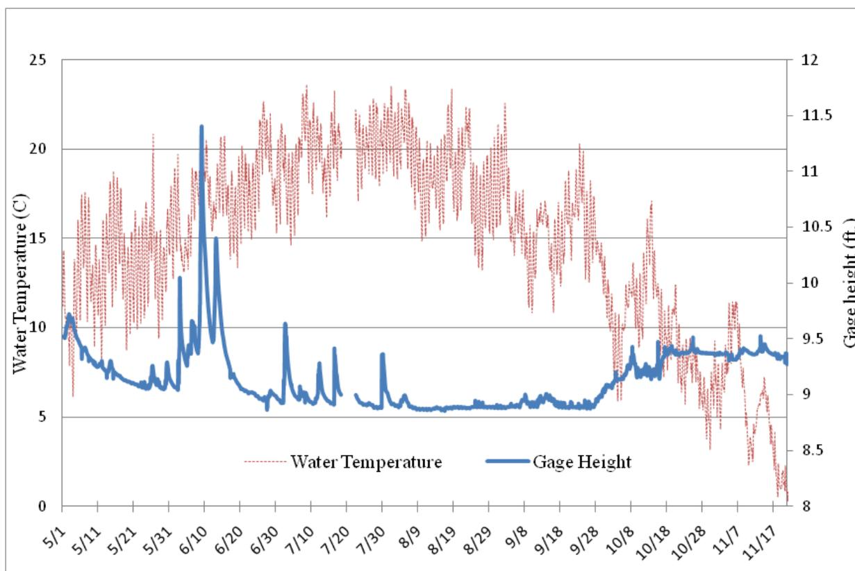
Figure 5.2. Gage height and water temperature for Trout Creek during May-November of 2008. Data was recorded at County Road FF using a datalogger, pressure transducer and thermocouple.
