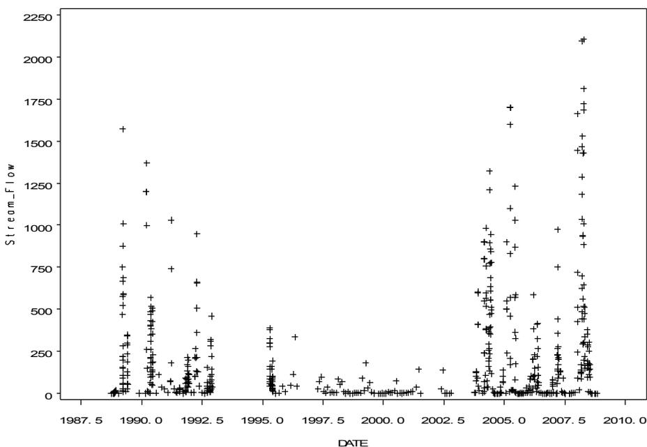
Figure 3.7. Measured stream flow (cfs) during phosphorus sampling from 1988-2008 at the Duck Creek USGS monitoring station. Three distinguishable periods are apparent, which coincide with different sampling protocols.
