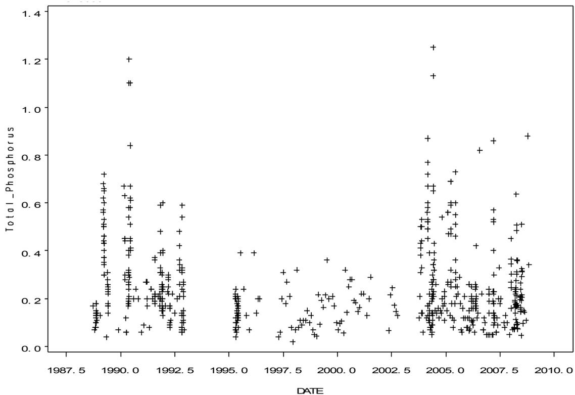
Figure 3.1. Distribution of total phosphorus concentrations (mg/L) in samples collected throughout the 20-year monitoring period (1988-2008). In years 1996-2002, sampling was primarily performed monthly, resulting in fewer samples and no samples of higher concentrations ( $>0.5$  mg/L).
