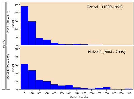
Figure 3.6. Histogram of stream flow during phosphorus sampling between periods one (1989-1995) and three (2004-2008). Proportionally fewer samples were taken at higher flows (>675 cfs) during Period 1, while fewer samples were collected at low flow (<75 cfs) during Period 3.
