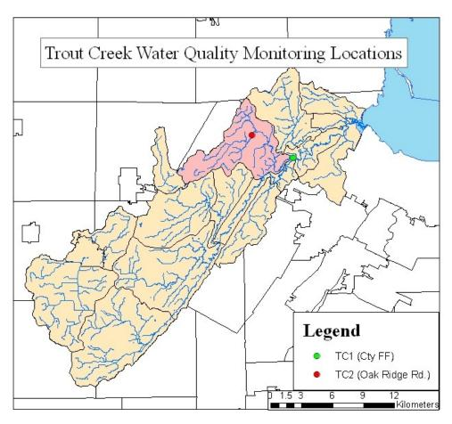
Figure 5.1. Location of the Trout Creek watershed and two water quality monitoring locations. Nutrient and physical water quality parameters were measured at TC1 (downstream) and TC2 (upstream) during 2008.
