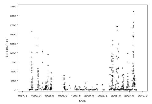
Figure 3.7. Measured stream flow (cfs) during phosphorus sampling from 1988-2008 at the Duck Creek USGS monitoring station. Three distinguishable periods are apparent, which coincide with different sampling protocols.
