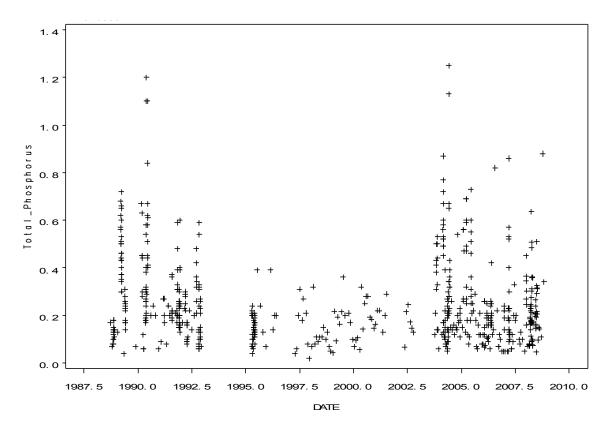
Figure 3.1. Distribution of total phosphorus concentrations (mg/L) in samples collected throughout the 20-year monitoring period (1988-2008). In years 1996-2002, sampling was primarily performed monthly, resulting in fewer samples and no samples of higher concentrations (>0.5 mg/L).
