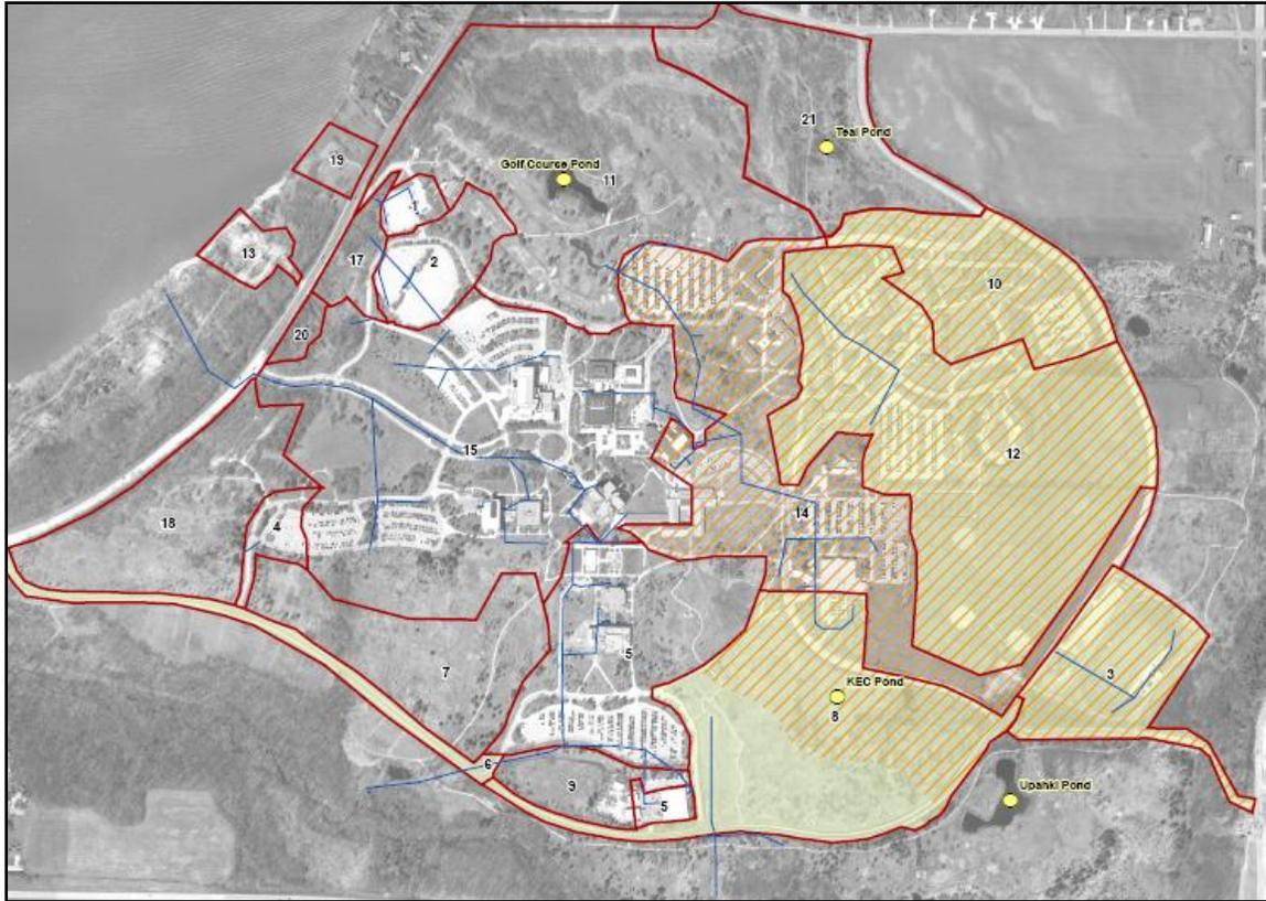
**Figure 3.1: Existing Stormwater BMPs and Drainage Basins as Identified by EarthTech (2008)**
