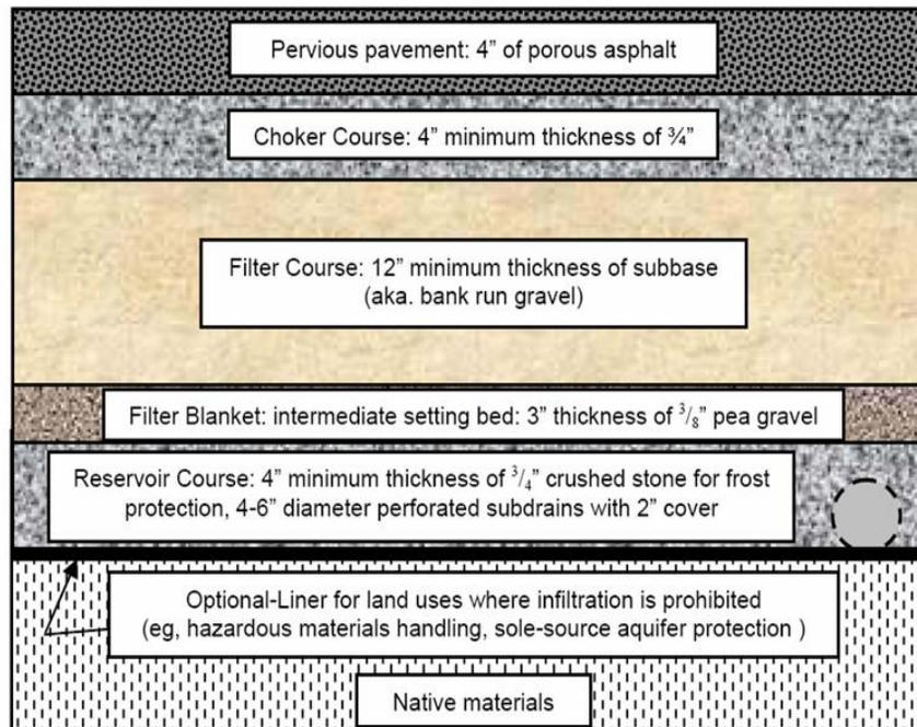
**Figure 3.7 Typical Cross Section of Pervious Pavement System (UNHSC 2008)**
