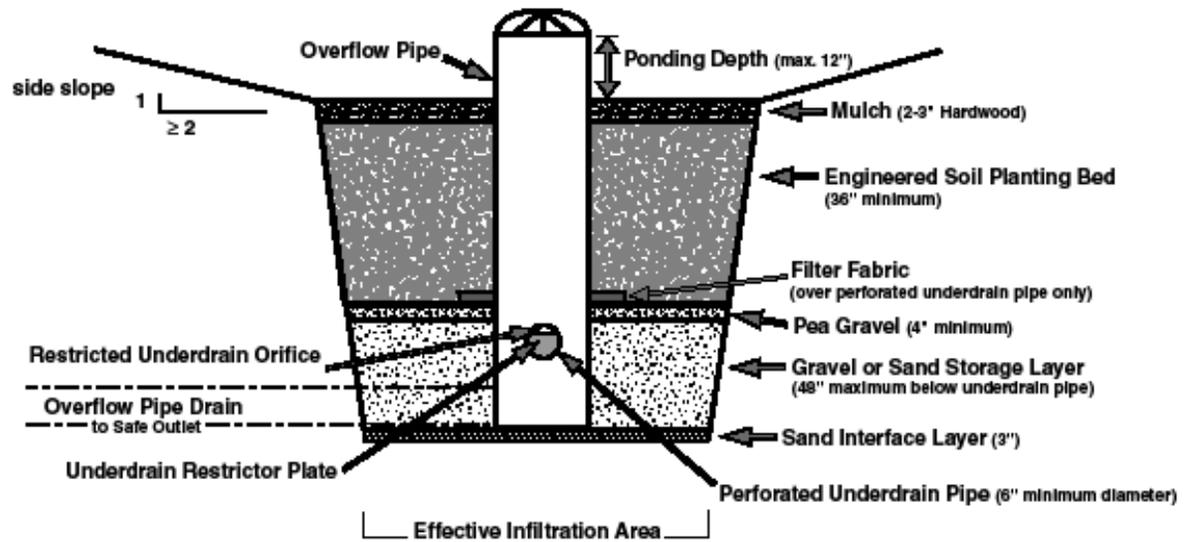
**Figure 3.6: Typical Components of a Bioretention Cell (WDNR 2006)**
