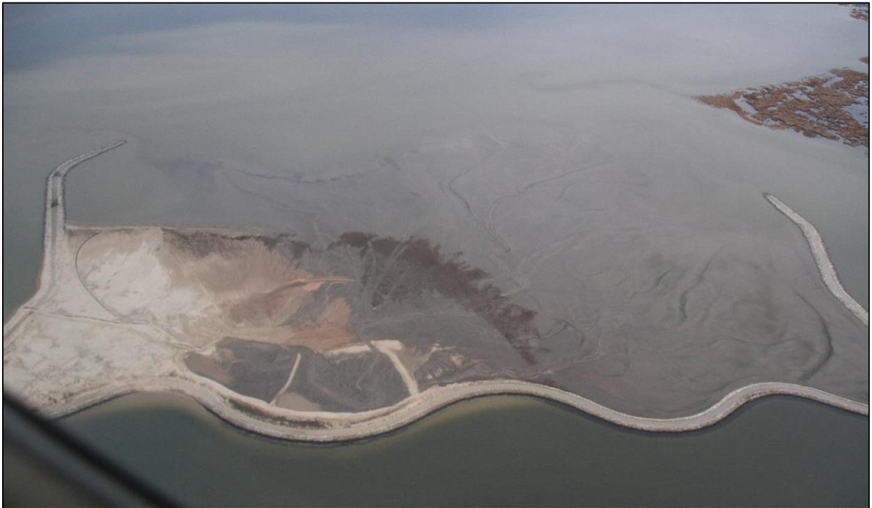
Photograph of the Cat Island Wave Barrier facing southwest, featuring the middle “cell,” which was recently filled with dredge material and historic Cat Island in the upper left. Photograph taken by Erin Giese on 2 December 2016.
